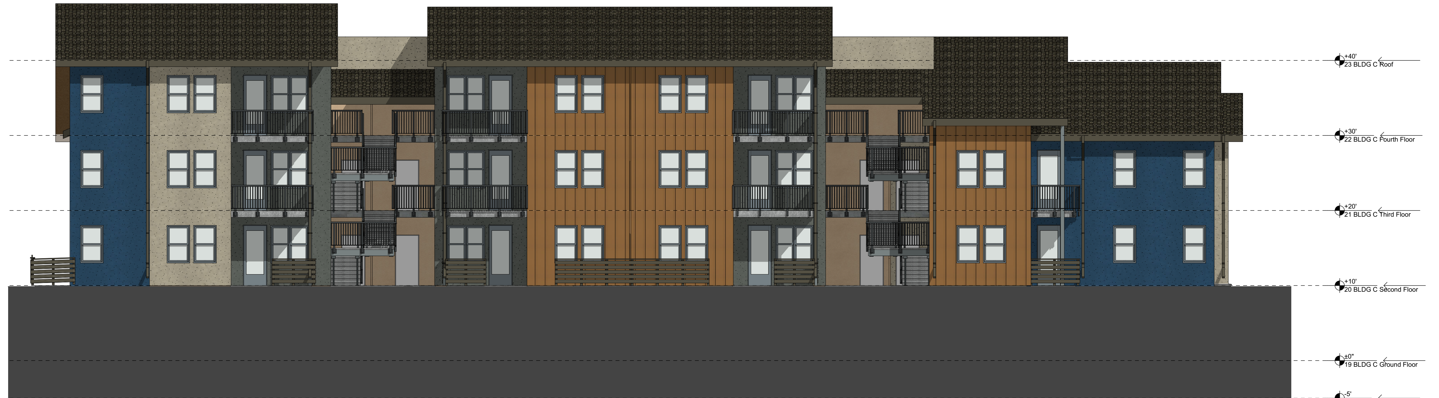
BLDG C NORTH ELEVATION - SCALE 1/8" = 1'-0"
