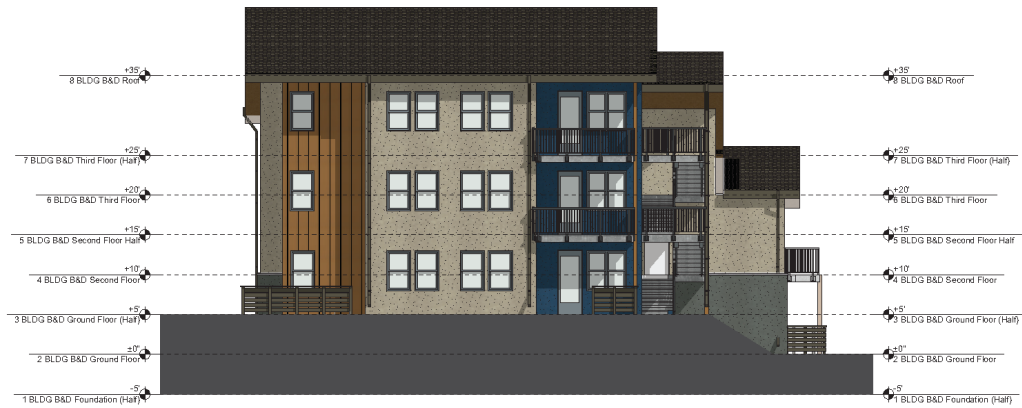
BLDG B NORTH ELEVATION - SCALE 1/8" = 1'-0"
